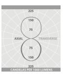
Luminaire Lumen Output 10W = 1455lm 20W = 2860lm
